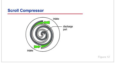
This orbiting motion causes the mated scrolls to form pockets of refrigerant vapor. As the orbiting motion continues, the relative movement between the orbiting scroll and the stationary scroll causes the pockets to move toward the discharge port at the center of the assembly, gradually decreasing the refrigerant volume and increasing the pressure.
